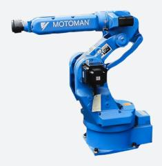
Capable of handling a wide variety of factory automation applications, the Motoman SK6 can also be used as an arc welder. The Motoman SK6 robot has six axes of motion and a durable cycloidal wrist design. Motoman SK6 features a maximum payload capacity of 6 kg and is fully functional with the MRC or the XRC Controller.
