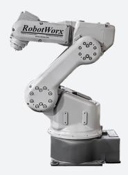
The Motoman SV3X features a 677 mm reach and offers the widest work envelope in its class. Six axes and a 3 kg payload make the SV3X XRC suitable for performing applications such as material handling, assembly, packaging, machine tending, and arc welding.
