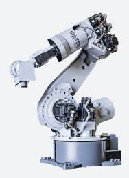
The six-axis Motoman ES165D "expert spot" welding robot provides fast, accurate, spot welding to users in all industries. Servo motors power the axes and arms of the ES165D to extend to a maximum 3,372 mm vertical reach and a 2,651 mm horizontal reach. The ES165D DX100 robot's axes have maximum speeds ranging from 110 degrees/second to 240 degrees/second, making it the fastest spot welding robot in the ES series. It is controlled by the Motoman DX100 controller and can manipulate up to 165 kg.
