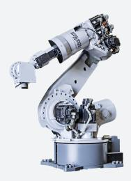
The Motoman ES165N "Expert Spot" robot is specifically designed to deliver unmatched performance and reliability in spot welding applications. To increase cable life, enhance safety, and reduce teaching time, the servo gun cables, air and water lines are routed through the ES165N's base and upper arm to the robot's wrist. The ES165N NX100 robot's compact, slim design allows it to reduce cycle time and reach into confined spaces, thus improving system productivity.
