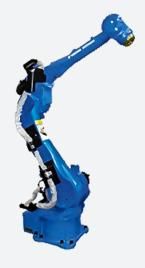
This compact Motoman MS80 offers numerous advantages as a spot welding robot. This robot produces fast movements, resulting in shorter cycle times and high throughput. Its smaller size allows it to be placed closer to the workpiece for added flexibility.
