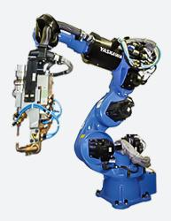
The VS100 is a great option for high-density layouts to help reduce cycle times as it provides a flexible reach and large range of motion with its seven degrees of freedom. This robot's slim design is flexible and beneficial for automotive applications as it can use DC spot guns with compact servo actuators. It can result in shorter production lines, the elimination of multiple stations, and tinier spot welding workcells as it can be placed in close proximity to other robots.
