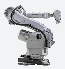
The Motoman UP165 sets the standard for versatility in the large robot marketplace. This high-speed robot offers a small footprint with superior performance in both spot welding and heavy payload handling applications. The UP165 XRC features and options include full 6-axis capability, application-specific software, Advanced Sigma motors to help provide a powerful and slim design, and a very wide working envelope of 2,650 mm (104.3") in reach.
