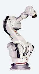
The Motoman UP200 is a fast, flexible, and powerful industrial automation robot. The UP200 robot offers minimal footprint and superior performance in both spot welding and heavy payload handling applications. With a 2,446 mm reach and the large payload of 200 kg, the Motoman UP200 XRC can achieve unmatched flexibility. The work envelope extends behind the body, allowing tools to be placed at the back and providing easy access to weld guns for maintenance.
