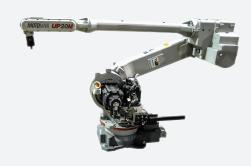
The Motoman UP20M XRC is a dynamic, flexible automation robot that offers quality arc welding, coating, dispensing, and material cutting applications. With a slim base, waist and arm design, the UP20M allows for close placement to workpiece holding fixtures thus improving part accessibility.
