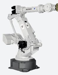
The Motoman UP350 is a heavy payload, high performance robot. It is a powerful addition to Motoman's extensive product line. Its hefty 350 kg payload and 2,542-mm reach provide versatility with heavy loads.
