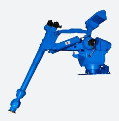
The highly flexible, six-axis, Motoman UP400RD II is the answer to your heavy duty material handling jobs. It can handle a payload of up to 400 kg, has a slim, space saving design, is shelf-mounted, and is energy efficient. Compared to previous models, the UP400RD II can save up to 70% on power consumption during motion and 25% during idle periods. The cables are guaranteed to last longer as they are routed through the robot base to the upper arm.
