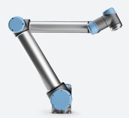
The UR10 is the largest robot in the Universal Robots collaborative series, with a payload up to 10 kg. It was built to conquer large tasks that still need great amounts of precision and reliability. The UR10 is the perfect collaborative choice for processes such as packaging, palletizing, assembly, and pick and place. It is effective at completing tasks across a larger area with a reach up to 1300 mm. This can save you time on production lines where distance can be a factor.
